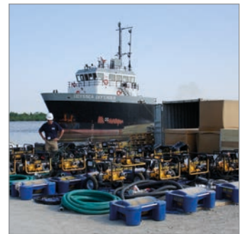
12. PD75s and skimmers being prepared for use on the Deepwater Horizon spill in the Gulf of Mexico.
